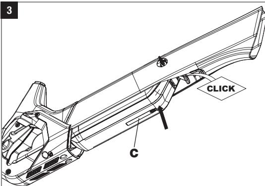
To completely lock the battery (C), apply pressure (upwards) to the battery pack in the area of the red retaining catch with lock. A "CLICK" sound is heard when the battery is securely locked into position.
