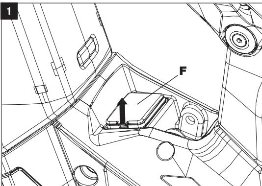
Open the cover (F) on the top of the motor interface by pulling on the small tab and flip it upwards.
