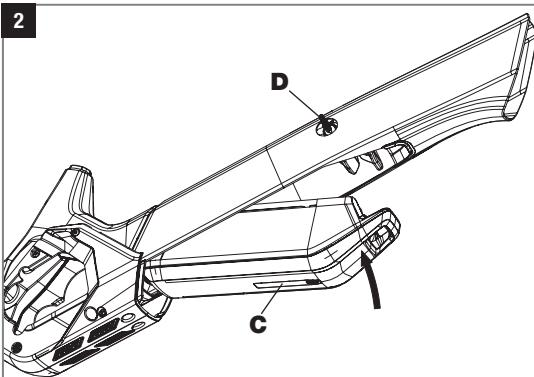
Now the battery (C) can be carefully guided upwards into the holder with lock.
