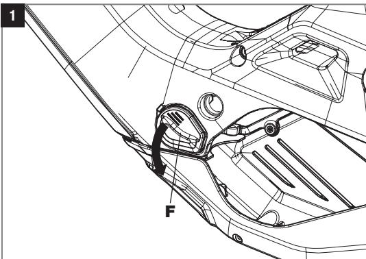
Unlock the cover (F) on the left-hand side of the motor interface with light pressure from above and turn it downwards to make the charging socket accessible.
