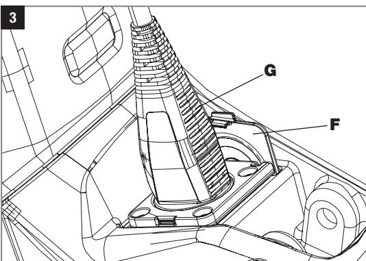
The charging socket is now accessible for the charging plug (G). Insert the charging plug (G) by applying light pressure. **The grooved side of the plug must point in the direction of the rear wheel and the side with the indentation towards the front wheel.** For details on how to charge the battery, please refer to the Bosch manual "Bosch eBike Battery Guide".
