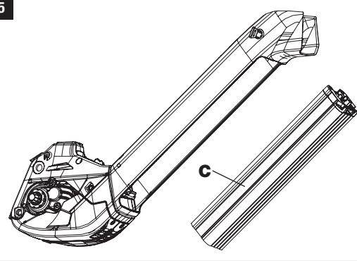
The battery (C) is now completely separated from the frame and can be transported for charging, for example.
