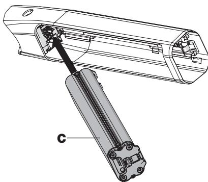
Carefully insert the battery (C) into the upper holder with lock.
