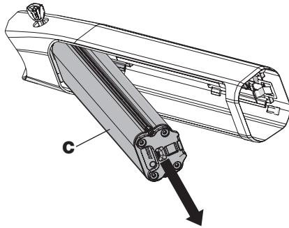
Next, pull the battery (C) downwards out of the holder.
