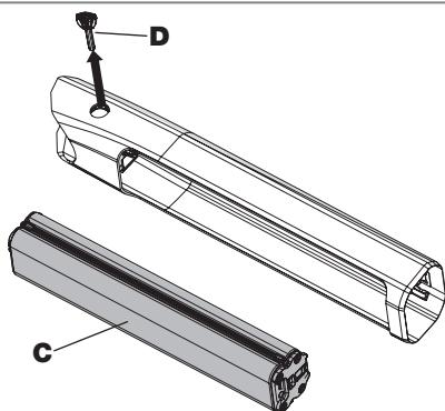
To install the battery (C), it must first be completely disconnected from the charger.
