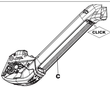
To completely lock the battery (C), apply pressure (upwards) to the battery pack in the area of the retaining catch with lock. A "CLICK" sound is heard when the battery is securely locked into position.
