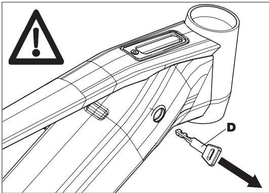
**The key (D) must be removed** before pedalling.
