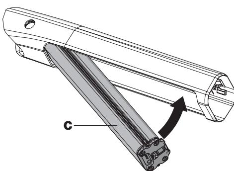
Next, carefully insert the battery (C) into the lower holder.
