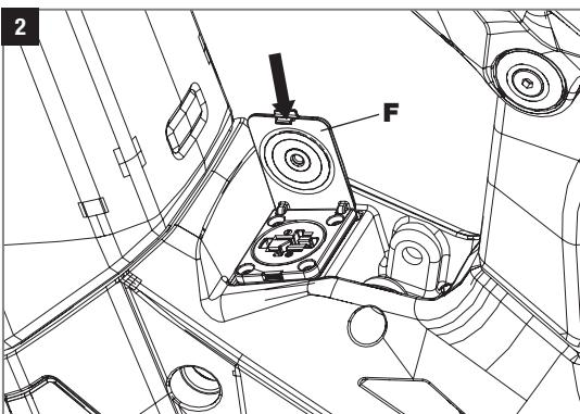
Slide the cover (F) with light pressure from top to bottom to ensure better access to the charging socket.
