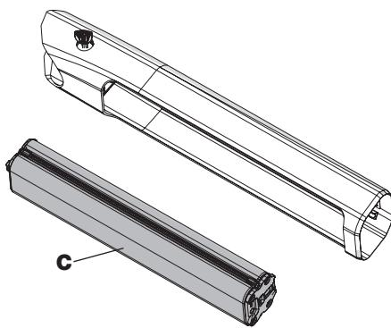
The battery (C) is now completely separated from the frame and can be transported for charging, for example.
