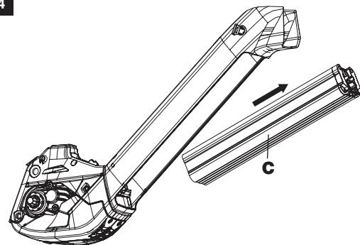
In the next step pull the battery (C) forward and out of the holder.
