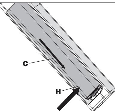
When the lock is opened, the battery (C) is released from the upper fixation and slides down a little. Continue to secure the battery by hand to prevent it from accidentally falling down (H).
