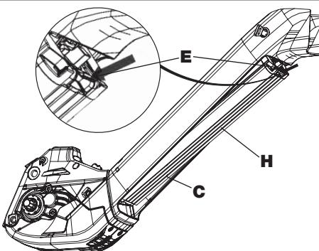
When the lock is opened, the battery (C) is released from the upper fixation. Continue to secure the battery by hand to prevent it from accidentally falling down (H).
