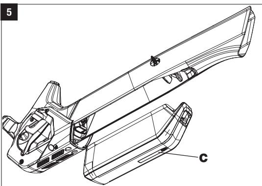
The battery (C) is now completely separated from the frame and can be transported for charging, for example.
