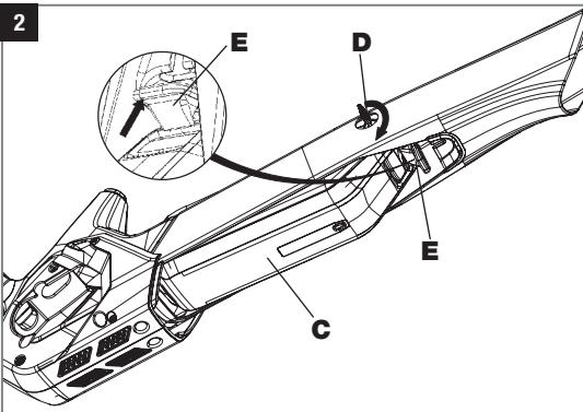
In the next step insert the key into the lock and turn the key clockwise to open the lock (D).
