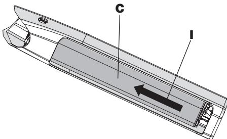
To fully secure the battery (C), push the battery in its current position slightly upwards (I) until you feel the battery click into place at the top and is fully fixed. The battery has now reached its final position.
