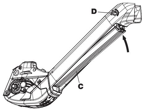
Now the battery (C) can be carefully guided upwards into the holder with lock.
