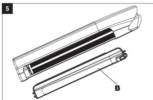
Slide the latch (A) down to release the lid (B) from its fixation. **2**
