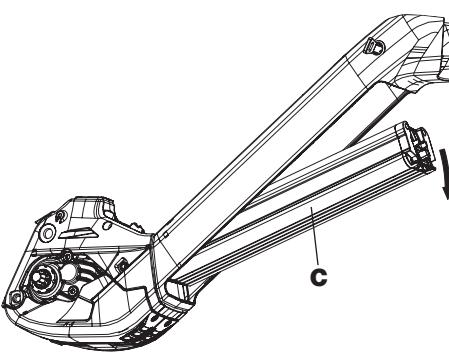
Hold the battery firmly with both hands so that it cannot fall out.
