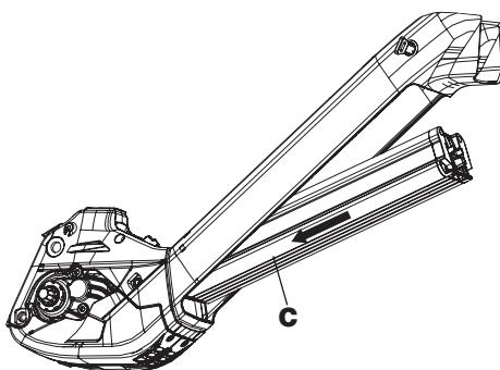
To install the battery (C), it must first be completely disconnected from the charger.
