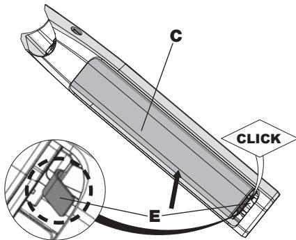
Insert the battery (C) into the lower holder until you hear a „CLICK“ sound from the fail-safe device (E).
