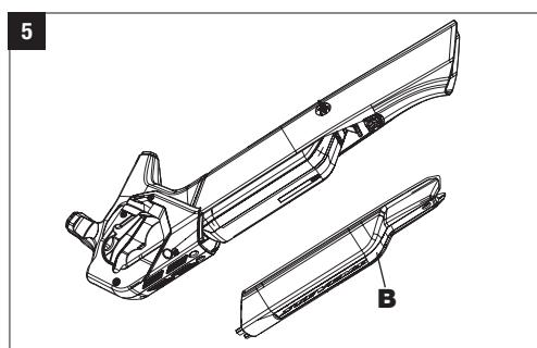
Press the button (A) to release the cover (B) from the fixation. **2**
