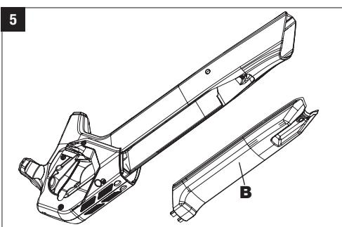
Press the button (A) to release the cover (B) from the fixation. **2**
