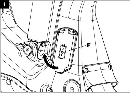
To open the cover (F) on the left side of the seat tube above the motor interface, apply light pressure to unlock it. Then lift it up slightly and carefully open it upwards.
