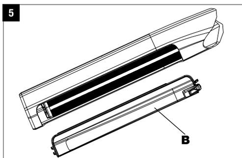
Slide the latch (A) down to release the lid (B) from its fixation. **2**
