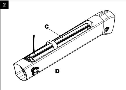
Now the battery (C) is carefully guided into the holder with the lock.
