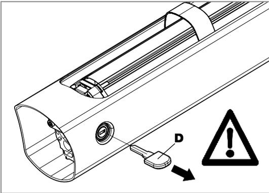
**The key (D) must be removed** before pedalling or turning the cranks. If the crank arm or the shoe touches the key during movement, the key, crank arm and lock may be damaged.
