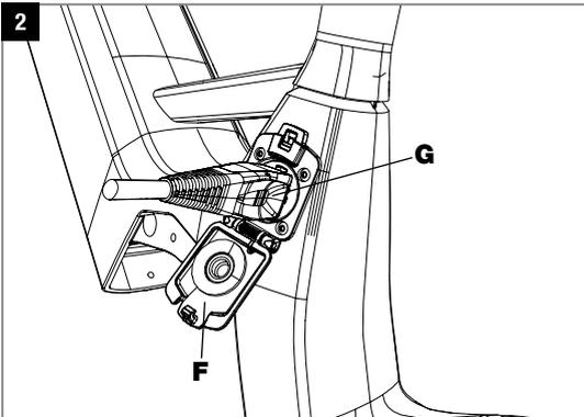
The charging socket is now accessible for the charging plug (G). Insert the charging plug (G) by applying light pressure. The grooved side of the plug must point in the direction of the front wheel and the side with the indentation towards the rear wheel. For details on how to charge the battery, please refer to the Bosch manual "Bosch eBike Battery Guide".
