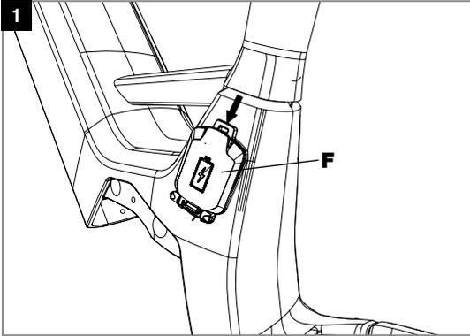
Remove the cover (F) on the left side of the seat tube above the motor interface by pressing the locking mechanism and open it downwards.
