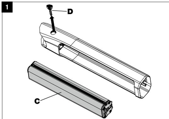
To install the battery (C), it must first be completely disconnected from the charger.
