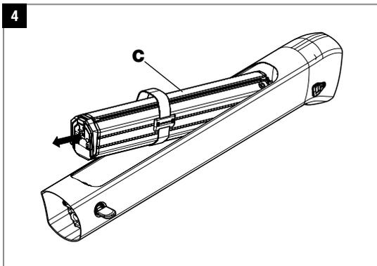
When removing, make sure that the battery (C) does not touch the seat tube, top tube or frame opening.
