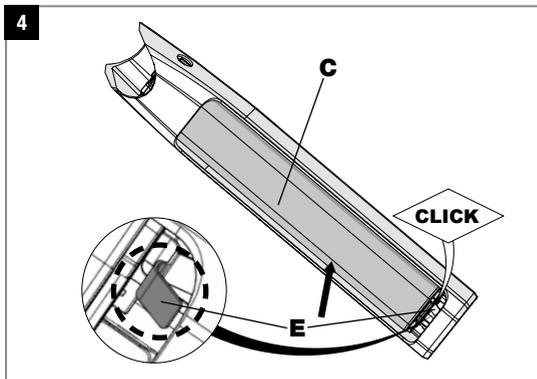
Insert the battery (C) into the lower holder until you hear a „CLICK“ sound from the fail-safe device (E).
