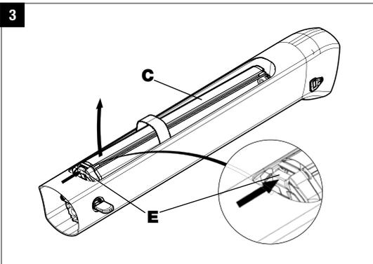
Be sure to first unlock the restraint system (E) with your finger. To do this, press it in the direction of the arrow. Then the battery (C) can be completely removed.
