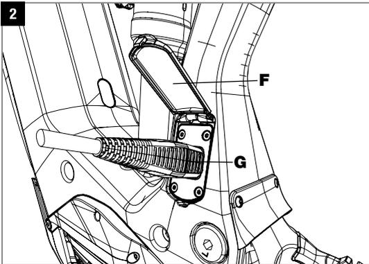
The charging socket can now be accessed with the charging plug (G). Insert the charging plug (G) by applying light pressure. The grooved side of the plug must point towards the rear wheel and the side with the indentation must point towards the front wheel. For details on how to charge the battery, please refer to the Bosch manual "Bosch eBike Battery Guide" or the STEVENS manual.
