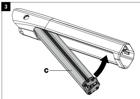
Next, carefully insert the battery (C) into the lower holder.
