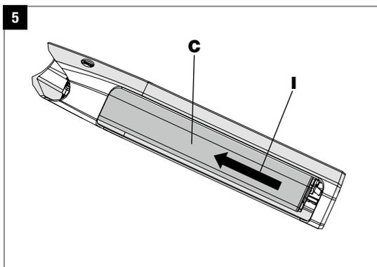
To fully secure the battery (C), push the battery in its current position slightly upwards (I) until you feel the battery click into place at the top and is fully fixed. The battery has now reached its final position.
