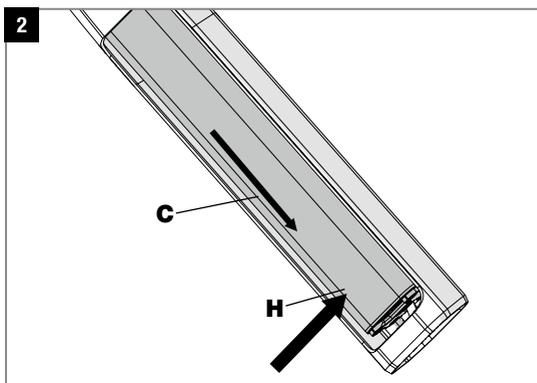
When the lock is opened, the battery (C) is released from the upper fixation and slides down a little. Continue to secure the battery by hand to prevent it from accidentally falling down (H).
