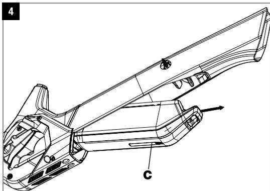
In the next step pull the battery (C) forward and out of the holder.
