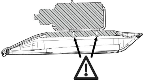
The threads for the bottle holder or accessories are **limited in how deep** they can go. A bolt can only be screwed **in to a certain depth**. The threads in the cap are M5 threads. If the screw is screwed in too far or tightened too much (MAX. 5 Nm), the cap, the thread or even the battery may be damaged. Please contact your STEVENS dealer to select the correct bolts.
