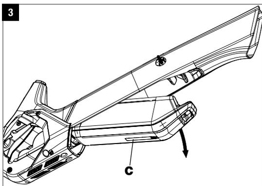
Now tilt the battery (C) downwards until it protrudes horizontally from the down tube.
