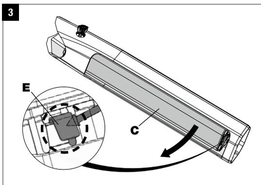
Press the retaining catch (E) in the direction of the motor to release the battery (C) from the holder. Hold the battery firmly with both hands so that it cannot fall out.
