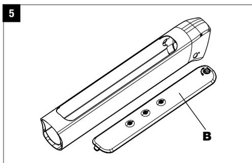
Turn the shutter (A) counterclockwise. This releases the cover (B) from the fixation. **2**
