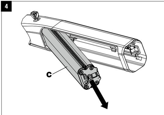
Next, pull the battery (C) downwards out of the holder.
