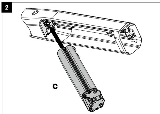
Carefully insert the battery (C) into the upper holder with lock.
