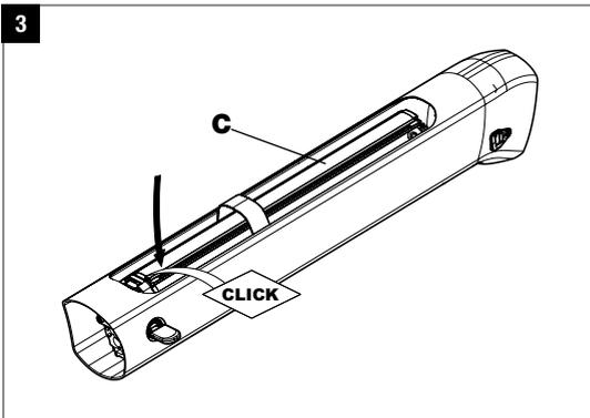
To ensure battery (C) is correctly locked into position, pressure (downwards) is applied to the battery in the area of the holder with lock. A "CLICK" sound is heard when battery is securely locked into position.
